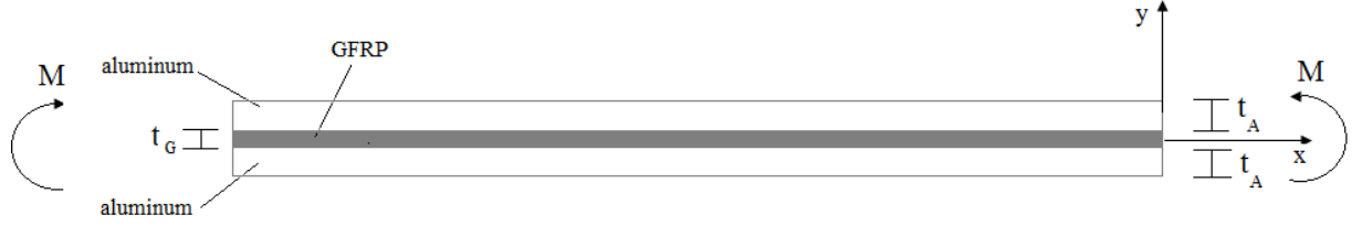
Figure 1: Three layers composite beam
