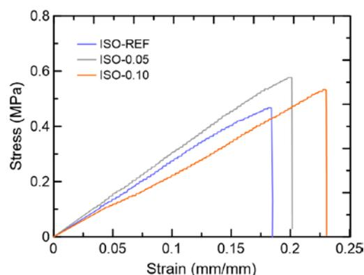
Figure 8: Influence of CNTs dosage on the tensile behavior of a cement paste
