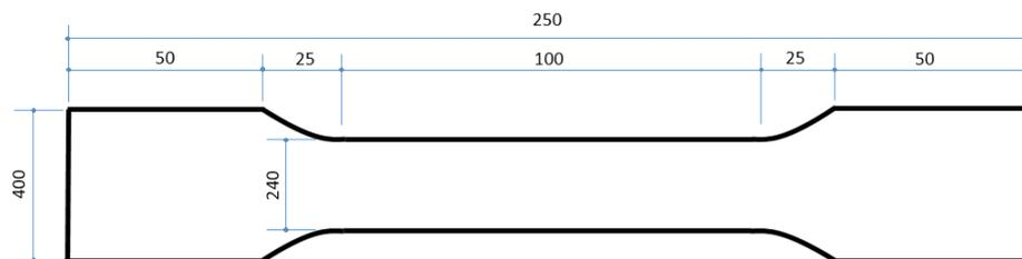
Figure 2: Specimen geometry used for tensile tests.
