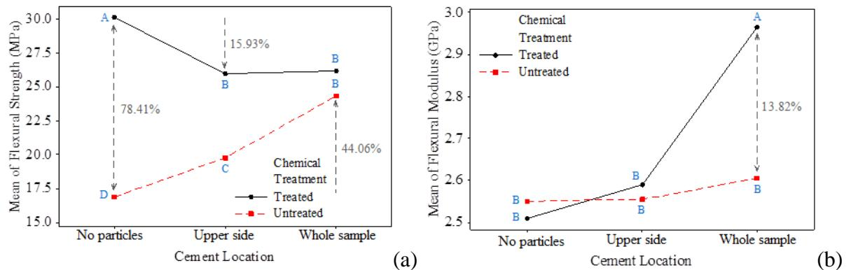
Figure 4. Effect plot for the mean responses: (a) flexural strength and (b) flexural modulus of the composites.
