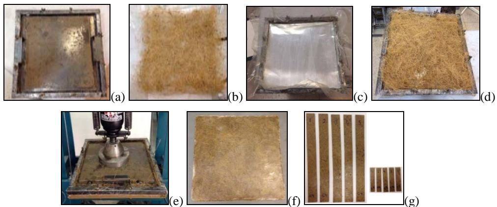
Figure 2. Fabrication process of the composites: (a) metallic mould, (b) fabric of random coir fibres, (c) aluminium plate, (d) fabric arranged inside the mould, (e) cold pressing, (f) composite plate and (g) specimens for testing.
