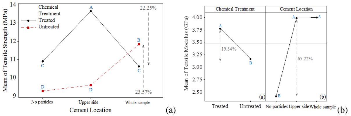
Figure 3. Effect plot for the mean: (a) tensile strength and (b) tensile modulus of the composites.
