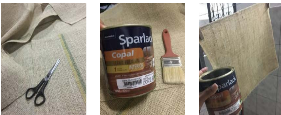
Figure 3 – Preparation and treatment with varnish (Polymeric Treatment) of fibre tissue.
