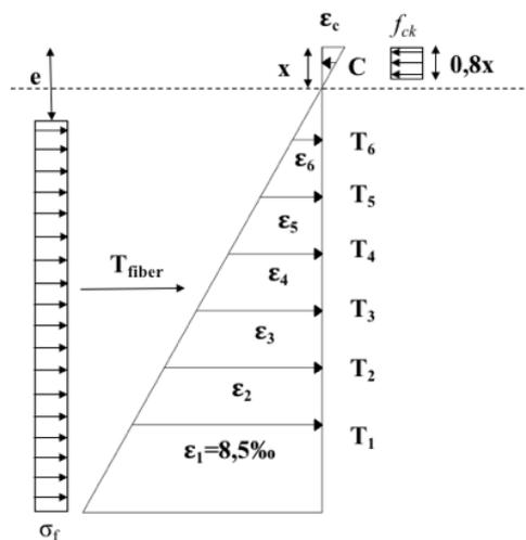
Figure 8. Force diagram for the sleepers with fibrous reinforcement
