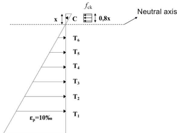
Figure 7. Force diagram for the sleeper without fibrous reinforcement
