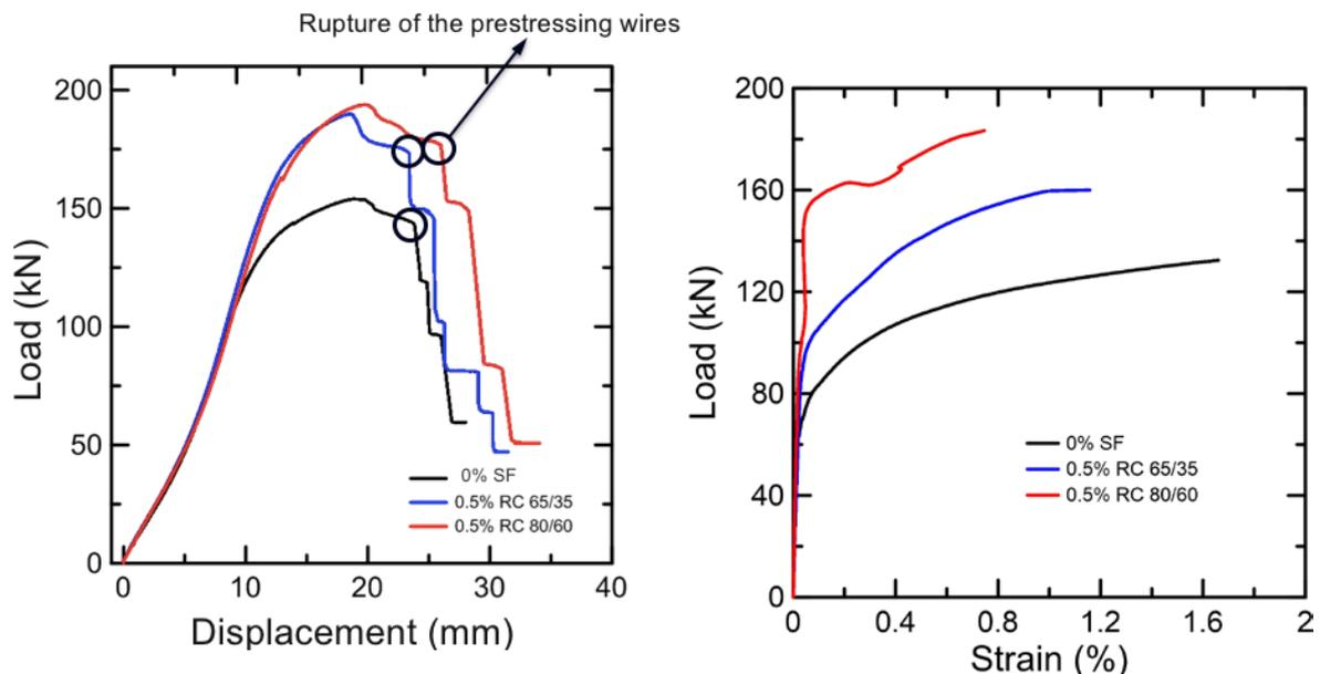
Figure 5. Load-Displacement and Load-Strain curves for each concrete mixture
