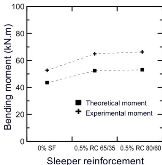
Figure 9. Comparative chart of bending moment values obtained by experimental test and theoretical calculations
