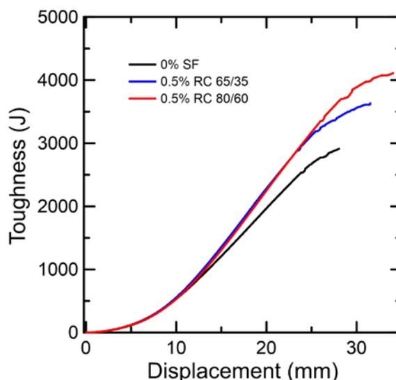
Figure 6. Toughness-Displacement curves for each concrete mixture
