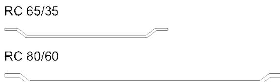
Figure 2. Geometry of the steel fibers used
