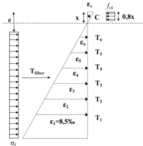
Figure 8. Force diagram for the sleepers with fibrous reinforcement
