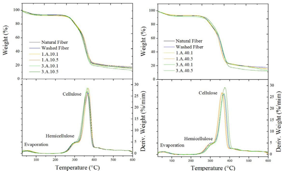
Figure 1: Thermogravimetry analysis (TG/DTG) of the sisal fibers before and after the different treatments.
