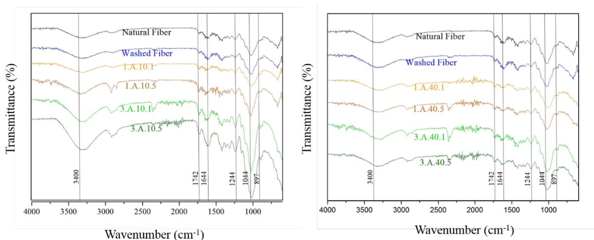
Figure 2: Infrared spectroscopy of sisal fiber before and after the different treatments.
