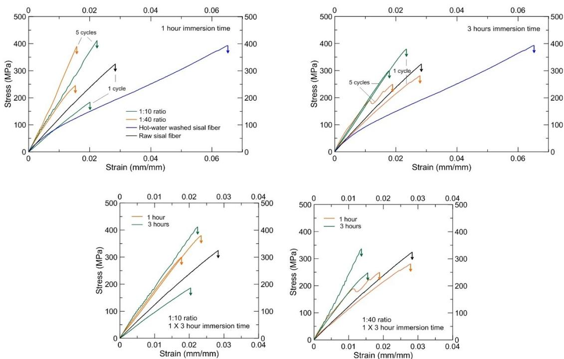
Figure 4: typical tensile curves of raw and treated fibres.
