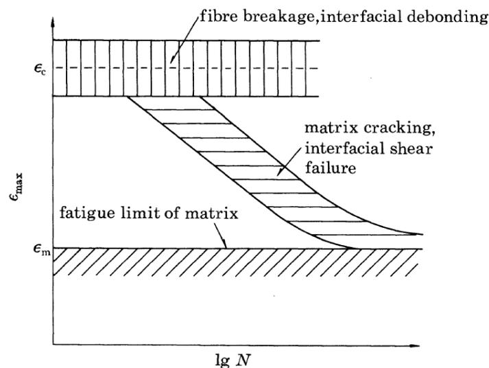
Figure 1: Fatigue life diagram for unidirectional composites [12]
