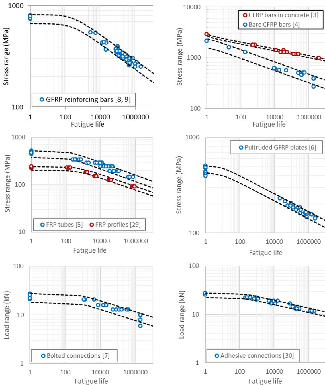
Figure 2: From top: calibrated models for a) GFRP reinforcing bars, b) CFRP reinforcing bars, c) GFRP coupons, d) pultruded GFRP plates, e) bolted connections, and f) adhesive connections
