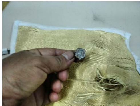
Figure 5- Fabric bulletproof sample after gunshot test
