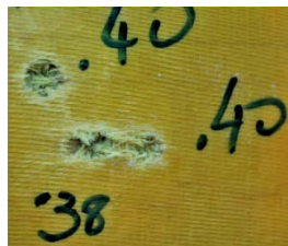
Figure 6 – Composite T3 after shotting test
