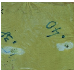
Figure 8 – Composite H1 after shooting test
