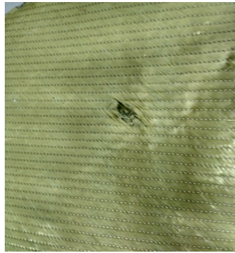
Figure 4- Bulletproof vest after gunshot test
