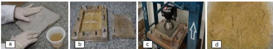
Figure 1: Manufacturing process of the hybrid composites: (a) lamination of the fibres, (b) wooden mould, (c) cold pressing, (d) material after compaction.
