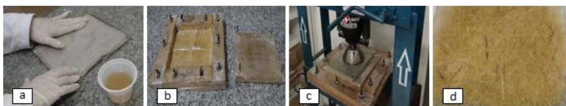
Figure 1: Manufacturing process of the hybrid composites: (a) lamination of the fibres, (b) wooden mould, (c) cold pressing, (d) material after compaction.
