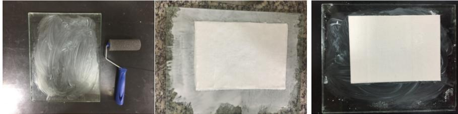
**Figure 2: Manufacturing process of composite materials.**
