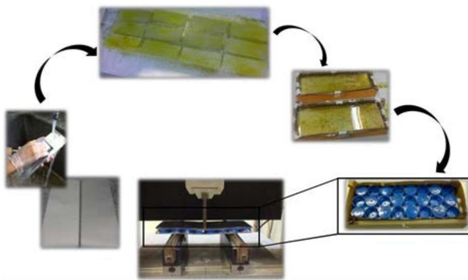
Figure 2: Sample manufacturing process based on surface treatment (a), preparation of the mould (b), bottle caps allocation (c), and finished sample during test (d).
