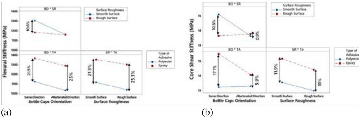
Figure 4: Interaction effect plot for flexural stiffness (a) and core shear stiffness (b).
