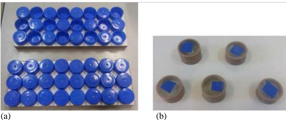
Figure 1: Alternated (above) and single directed (below) bottle caps configurations (a) and micro-hardness bottle caps samples (b).
