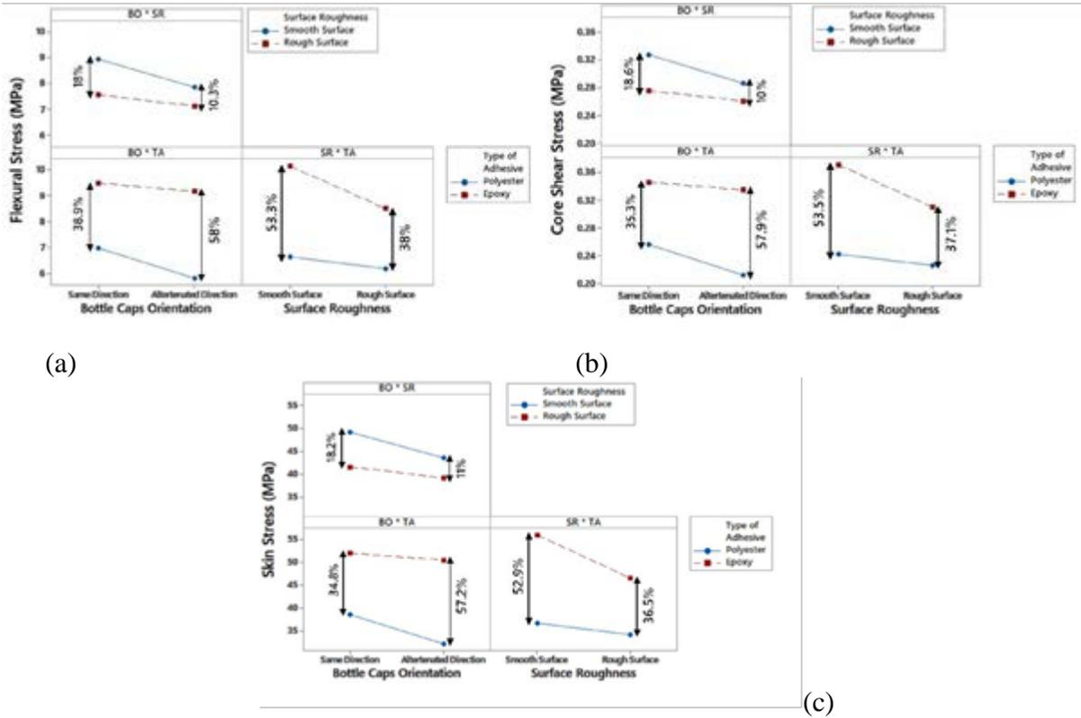
Figure 3: Interaction plot for flexural stress (a), core shear stress (b) and skin stress (c).
