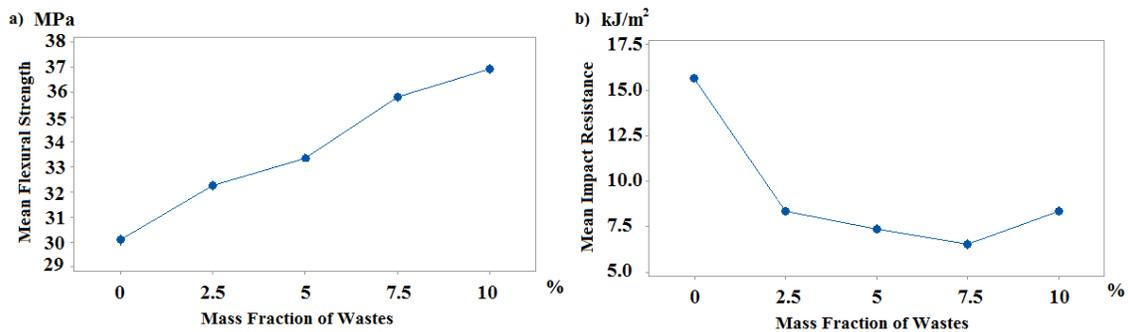
Figure 6 – Main effect plot for (a) mean flexural strength and (b) impact resistance.
