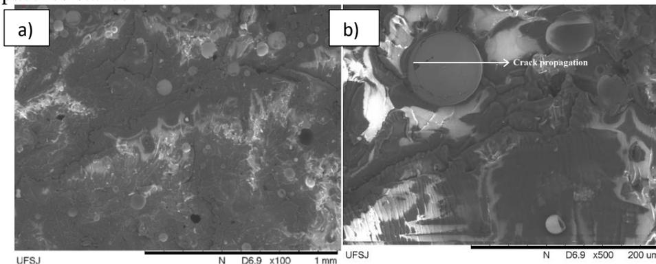
Figure 8 - BSE image: a) Fractured region of tensile test specimen with 10% waste incorporation, magnified 100 times. b) Tensile test fracture surface of a specimen with 10% of waste, magnified 500 times.
