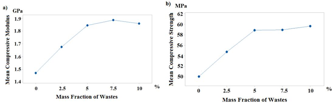
Figure 5 - Main effect plot for mean compressive (a) modulus and (b) strength.
