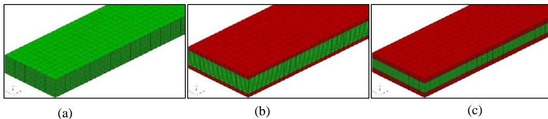
Figure 2: Discretization by finite elements of (a) polymer epoxy, (b) PE3L and (c) PE5L
