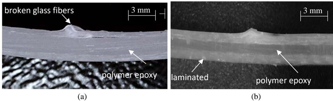
Figure 4 : Failure modes in the polymer epoxy reinforced with (a) 3 and (b) 5 layers of glass fiber laminated
