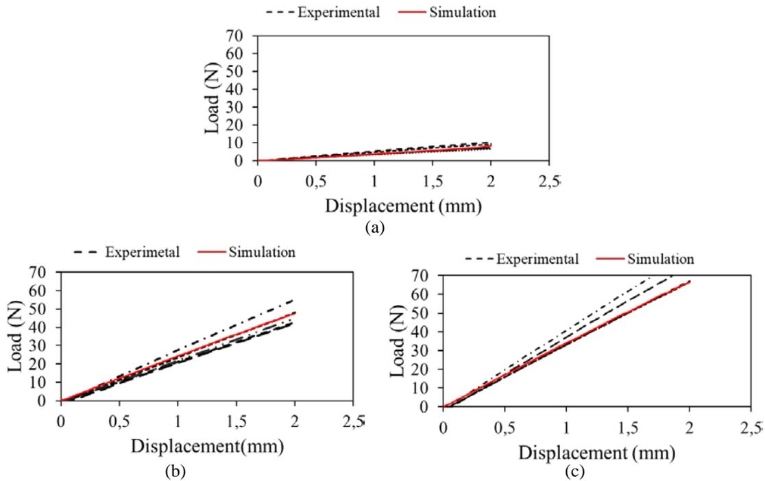
Figure 6: Load x Displacement diagram of flexural tests by experimental and numerical simulation: (a) Polymer Epoxy, (b) PE3L and (c) PE5L
