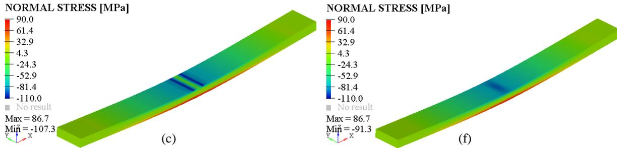
Figure 5: Linear simulation results of (a) polymer epoxy (b) PE3L and (c) PE5L. Non-linear simulation results of (d) polymer epoxy (e) PE3L and (f) PE5L.
