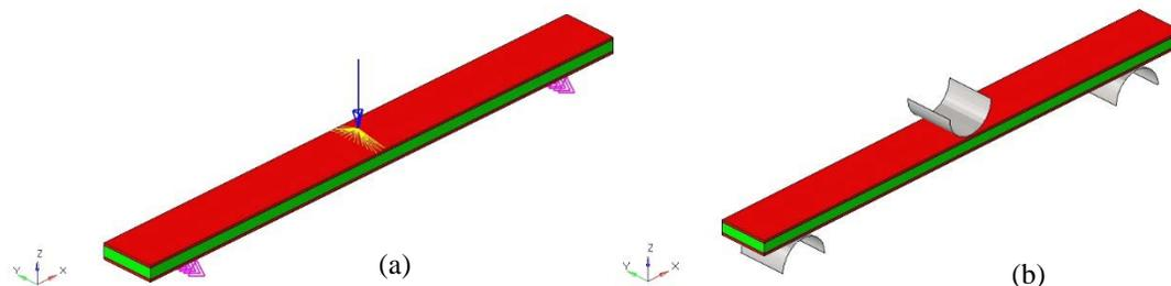
Figure 3: (a) Rigid elements and constrains used in linear simulation and (b) cylindrical support surface used in non-linear simulation
