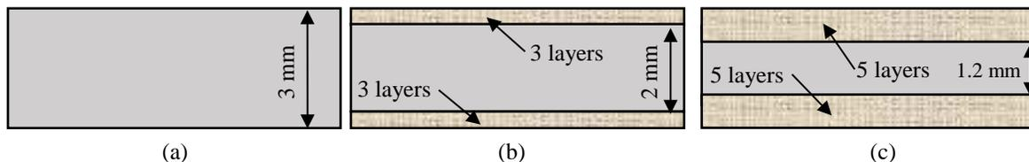
Figure 1: Sample illustration: (a) polymer epoxy, (b) PE3L and (c) PE5L
